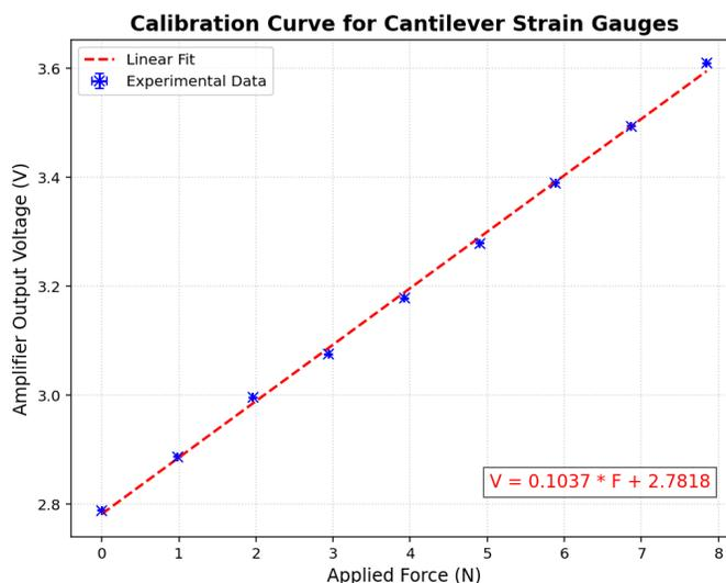
Figure 11: Calibration curve, corresponding to data seen in Table 7 - showing relationship between output voltage versus Force
