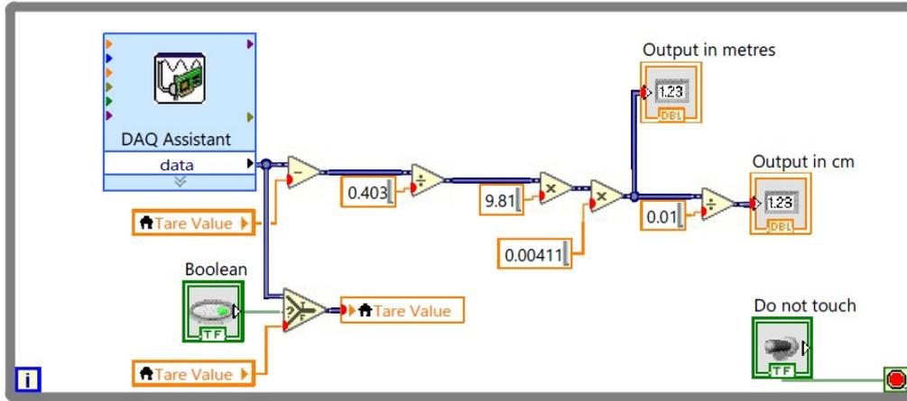
Figure 10: Tare mechanism implemented in LabView
