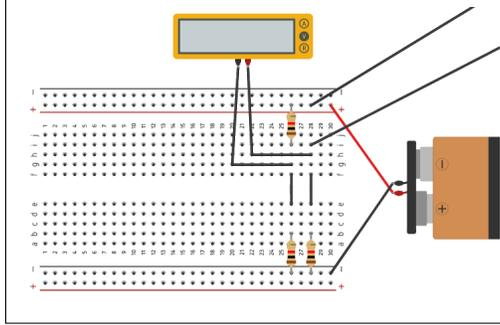
Figure 1: Current Wheatstone Bridge Set-up
