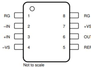
Figure 2: INA122P Pin Diagram
